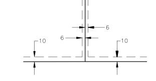
BEING 6 FEET IN WIDTH AND ADJOINING LOT LINES AND BEING 10 FEET IN WIDTH AND ADJOINING RIGHT-OF-WAY LINES, UNLESS OTHERWISE INDICATED ON THE PLAT.
